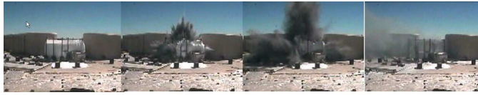
Figure 4: A modern implosion experiment carried out at the dual axis radiographic hydrodynamic test facility at LANL. High energy x-rays interrogate the object as it implodes.
